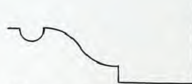
No. 933.—Angle moulding ; any size to suit.
